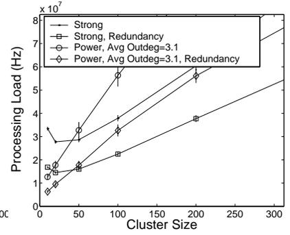
Figure 6: Individual processing load increases with cluster size
