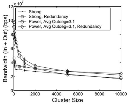
Figure A-13: Aggregate load with lower query rate
