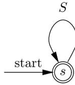
Fig. 10.44. Automaton with only the start state.
