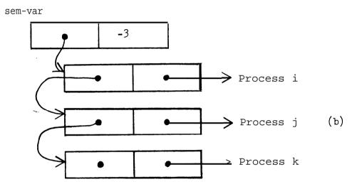
Figure 2: (a) No processes waiting (b) Three processes suspended
