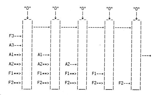
Fig.3 A Six-input, Five-level Signature Table Arrangement
