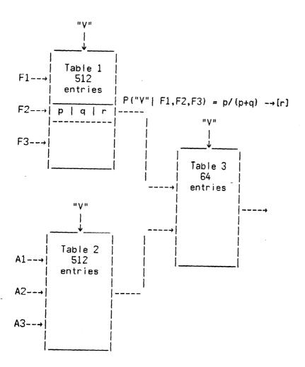
Fig.1 A Simplified Example of a Two-level Signature Table Arrangement Used in the Speech Recognition Program [2].
