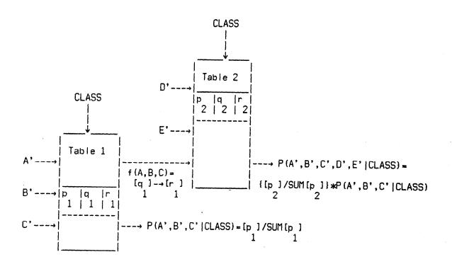
Fig. 2. A Simplified Two-level Signature Table Arrangement
