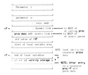
If a formal parameter is a value parameter, then the actual parameter value is kept on the stack. If a formal parameter is a reference parameter, then the
