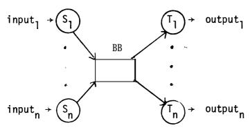
Process  $S_i$  reads an input stream,  $input_i$ , of m elements and feeds them into a bounded buffer BB.  $T_i$  removes m elements from the buffer (not necessarily the m elements appended by  $S_i$ ) attd prints them on  $output_i$ . One can prove
