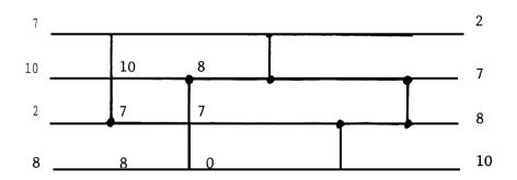
Figure 4. For input vector  $\vec{x} = \langle 7, 10, 2, 8 \rangle$ , one has  $\vec{x}^{(1)} = \langle 2, 10, 7, 8 \rangle$ ,  $\vec{x}^{(2)} = \langle 2, 8, 7, 10 \rangle$ , and output  $\vec{x}\alpha = \vec{x}^{(4)} = \langle 2, 7, 8, 10 \rangle$ .
