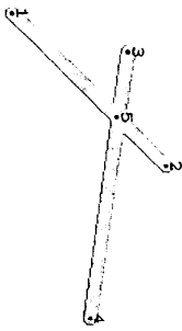
Fig. 5-1. The coordinates of point 5 can be readily calculated from those of points 1, 2, 3, and 4, using METAFONT equations.
