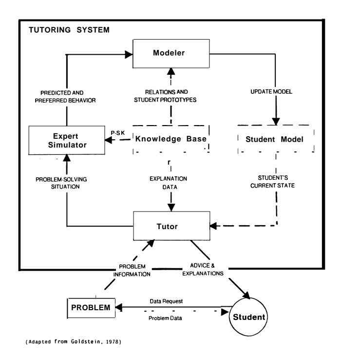
Figure 1-1: Components of an ITS
