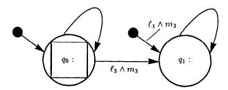
This automaton has two states, the good state  $q_0$  associated with the condition  $\neg(\ell_3 \land m_3)$ , and the bad state  $q_1$ , to which we switch on detection of a program state satisfying  $\ell_3 \land m_3$ . Once we are in  $q_1$  we can never get out.
