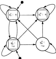
Following the syntax of State&arts [Hal], we introduce two additional conventions that lead to more compact and structured representation of diagrams. We introduce the notion of *super-states* represented as boxes containing other states. As a general rule we interpret any construct associated with a super-state to be associated with every contained state. The two applications of this general rule are:
