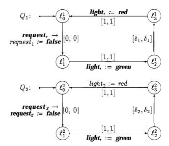
If the combined traffic light controller makes use of **two** processors and the processes  $Q_1$  and  $Q_2$  are executed in a truly concurrent fashion, then the correctness of the entire system
