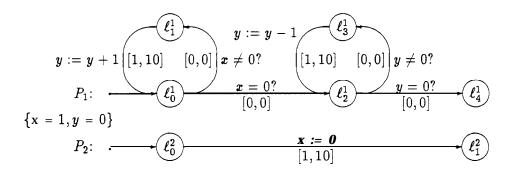
We wish to analyze the worst-case (maximal) running time of the synchronous two-process shared-variables multiprocessing system
