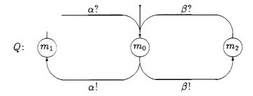
(Recall that we may omit the data components of message-passing operations, if they are immaterial.) The arbiter Q mediates between the two processes  $P_1$  and  $P_2$  and uses synchronous communication on the two channels  $\alpha$  and  $\beta$  to ensure mutual exclusion:  $P_1$  and  $P_2$  can never be simultaneously in their critical sections  $\ell_1^1$  and  $\ell_2^2$ , respectively.
