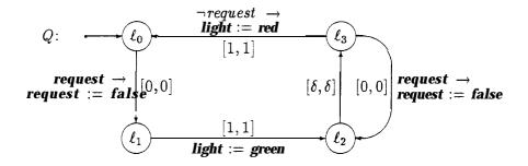
for any delay  $4 \le \delta \le 23$ . This implementation of the traffic light controller turns the light green as soon as possible after a request is received and then waits for  $\delta$  time units before turning the light red again. Only if the request button has been pushed in the meantime, the light stays green for another  $\delta$  time units.
