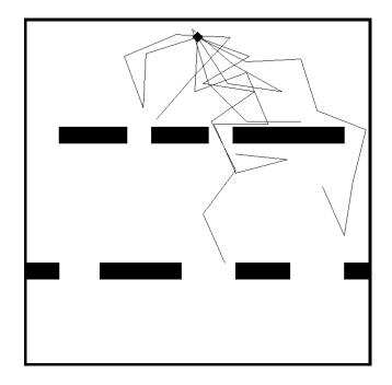
Figure 1: Several configurations of a robot with 7 degrees of freedom. This robot arm has 7 articulated joints, and must maneuver through gaps in two walls.
