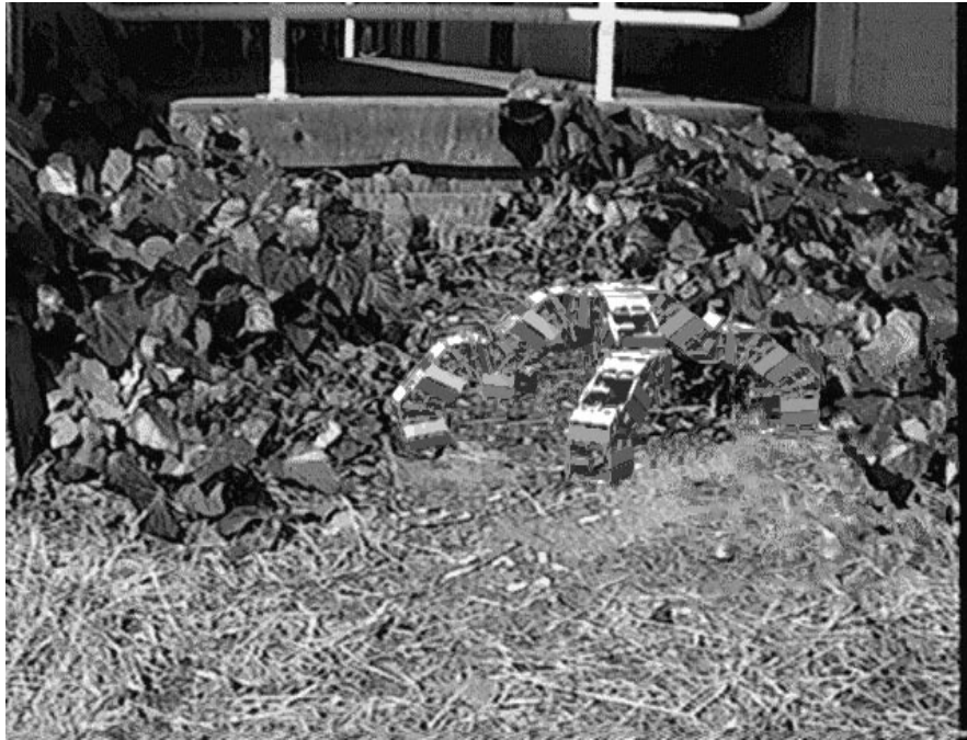
Figure 6.10: Polypod using the spider gait on rough earth
