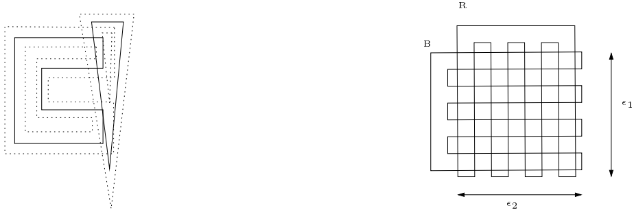
Figure 1: a) Intersection of two toleranced polygons and (b) Worst-case example of intersection
