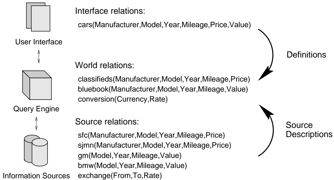
Figure 6.2: The information integration problem is abstracted as describing the relationships between three kinds of relations: Interface relations conceptualize the interaction with a user through a WWW based user interface. Source relations represent the data that is actually stored in the available information sources. World relations are used as means to describe both interface and source relations and are crucial in the query planning process.
