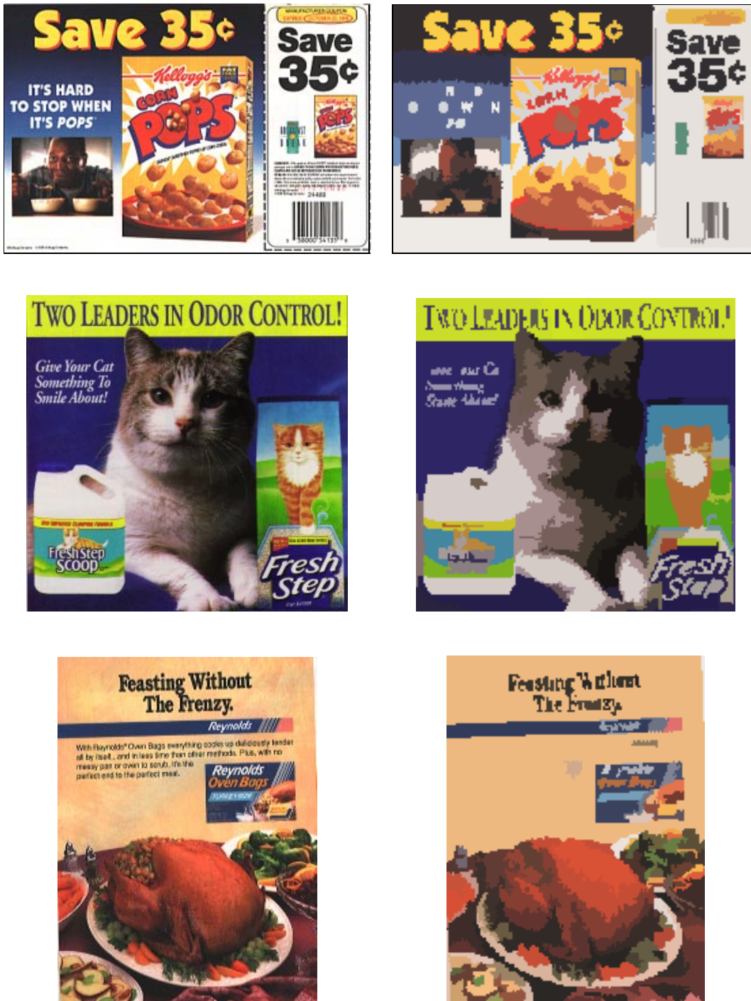
Figure 7.12: Region Merging Results. (left) Original image. (right) The original image reduced to 128 regions. Each region is colored with the average color of its pixels.
