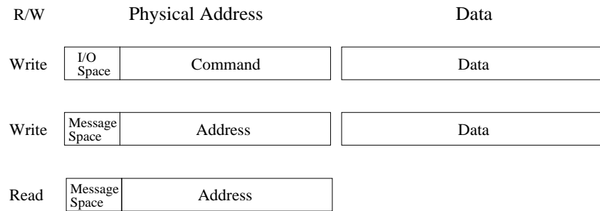
Figure 5: Processor to PP command formats.
