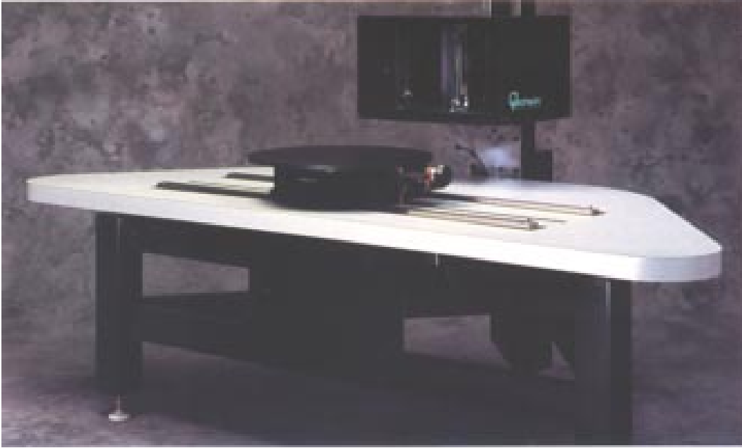
Figure 1.5: A photograph of the Cyberware Model MS 3030 optical triangulation scanner used for acquiring range images in this thesis.
