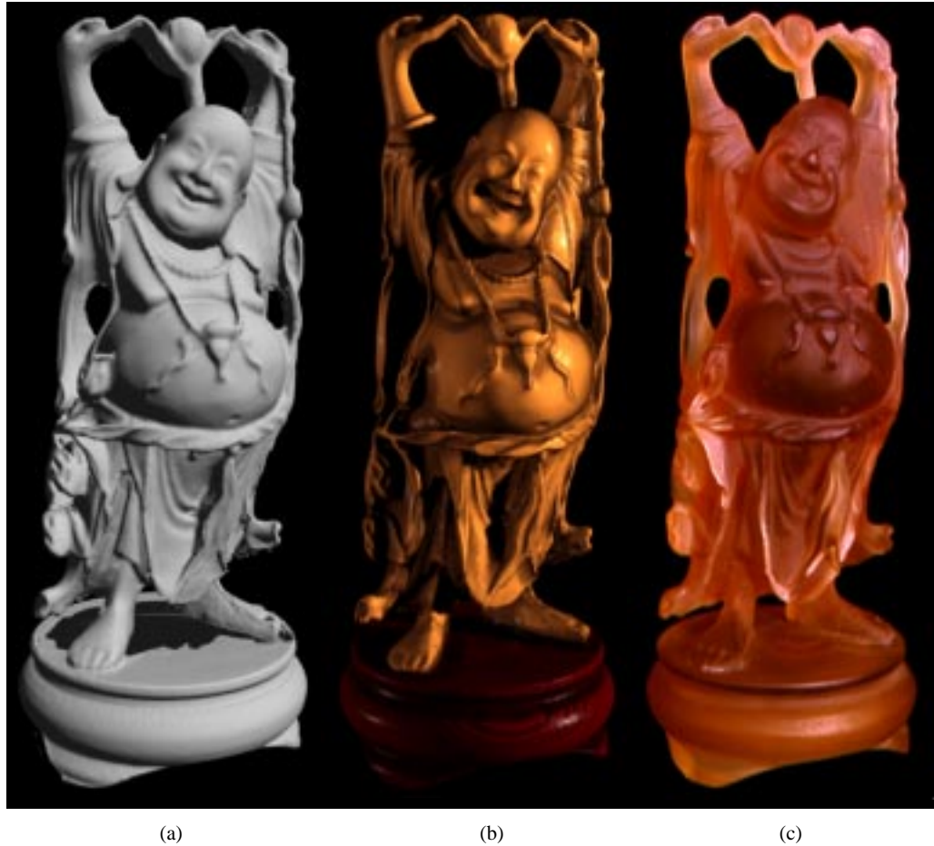
Figure 8.6: From the original to a 3D hardcopy of the “Happy Buddha” – Part II of II. (a) Gouraud-shaded rendering of the 2.4 million polygon mesh after merging 48 scans, but before hole-filling. Notice that the reconstructed mesh has at least as much detail as the single range image, but is less noisy; this is most apparent around the belly. The hole in the base of the model corresponds to regions that were not observed directly by the range sensor. (b) RenderMan rendering of an 800,000 polygon decimated version of the hole-filled and filtered mesh built from 58 scans. By placing a backdrop behind the model and taking 10 additional scans, we were able to see through the space between the base and the Buddha’s garments, allowing us to carve space and fill the holes in the base. (c) Photograph of a hardcopy of the 3D model, manufactured by 3D Systems, Inc., using stereolithography. The computer model was sliced into 500 layers, 150 microns apart, and the hardcopy was built up layer by layer by selectively hardening a liquid resin. The process took about 10 hours. Afterwards, the model was sanded and bead-blasted to remove the stair-step artifacts that arise during layered manufacturing.
