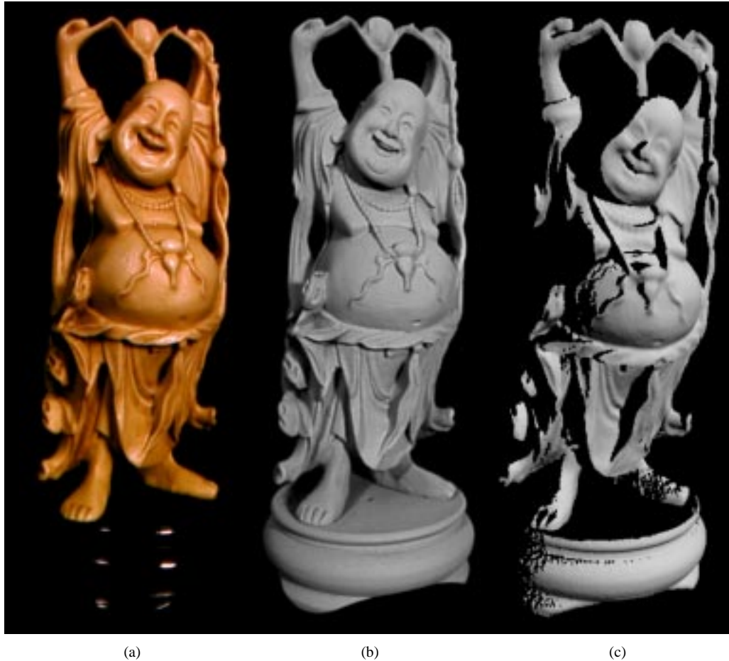
Figure 8.5: From the original to a 3D hardcopy of the “Happy Buddha” – Part I of II. (a) The original is a plastic and rosewood statuette that stands 20 cm tall. (b) Photograph of the original after spray painting it matte gray to simplify scanning. (c) Gouraud-shaded rendering of one range image of the statuette. Scans were acquired using a Cyberware scanner, modified to permit spacetime triangulation. This figure illustrates the limited and fragmentary nature of the information available from a single range image.
