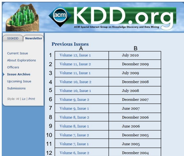
Figure 2: Web page from SIGKDD Explorations. HTML <TABLE> tags are the structure for the list of issues (A) and publication dates (B), denoted by solid lines (1–12)
