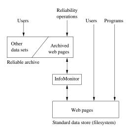
Fig. 2. The architecture of our implemented InfoMonitor system.
