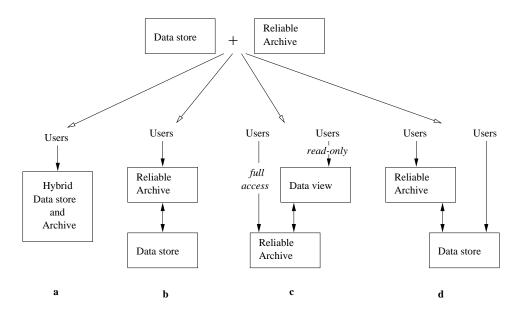
Fig. 1. Options for combining an existing data store with an archival component.
