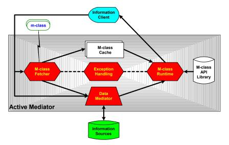
**Figure 3: Active Mediation Architecture**
