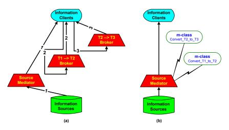
**Figure 5: Type Conversion for Autonomous Services**
